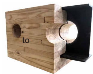
■ Steel perforated beam fireproofed with wood
