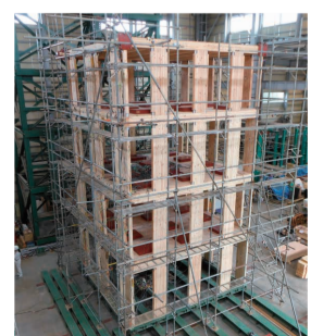
Four-story full-scale load test
